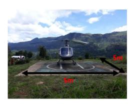
When directing helicopter to land stand at edge of cleared area with back to wind. Stay in pilot's vision. Ensure sufficient area cleared for main and tail rotor. Wear brightly colored clothing so that you are easily seen.
